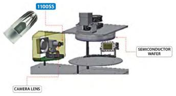
AFTER EXAIR: EXAIR recommended air cleaning with the Model 1100SS Super Air Nozzle. The reason is to create a non-contact wiping; so that, there is no need to purchase cleaning chemicals and it is no longer necessary to replace the camera lens due to abrasions from wiping. Labor costs reduced because manual lens cleaning was no longer required. A more reliable machine with less maintenance makes it a more attractive purchase for customers.
