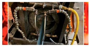
A producer of custom products needs to reduce compressed air consumption and noise levels associated with the use of coolant hose and copper tubing in a rollform blow off application.
