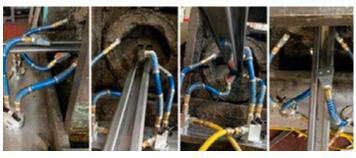
AFTER EXAIR: A Two Model 1100 Super Air Nozzles and two Model 1122 2" Flat Super Air Nozzles were purchased and installed (above) using Model 9043 Magnetic Bases and Model 9212 12" Stay Set Hoses. Coolant and debris were still effectively removed from the product. Compressed air consumption and noise levels dropped to 86.8 SCFM @100 PSIG, and 83.8 dBA, respectively.
